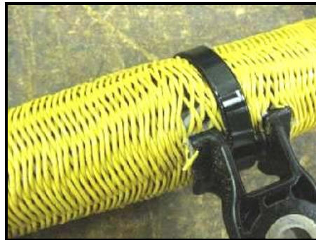
Fig. 15: Saddle Clip after Vibration Testing
